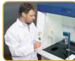
Tracer gas containment test
